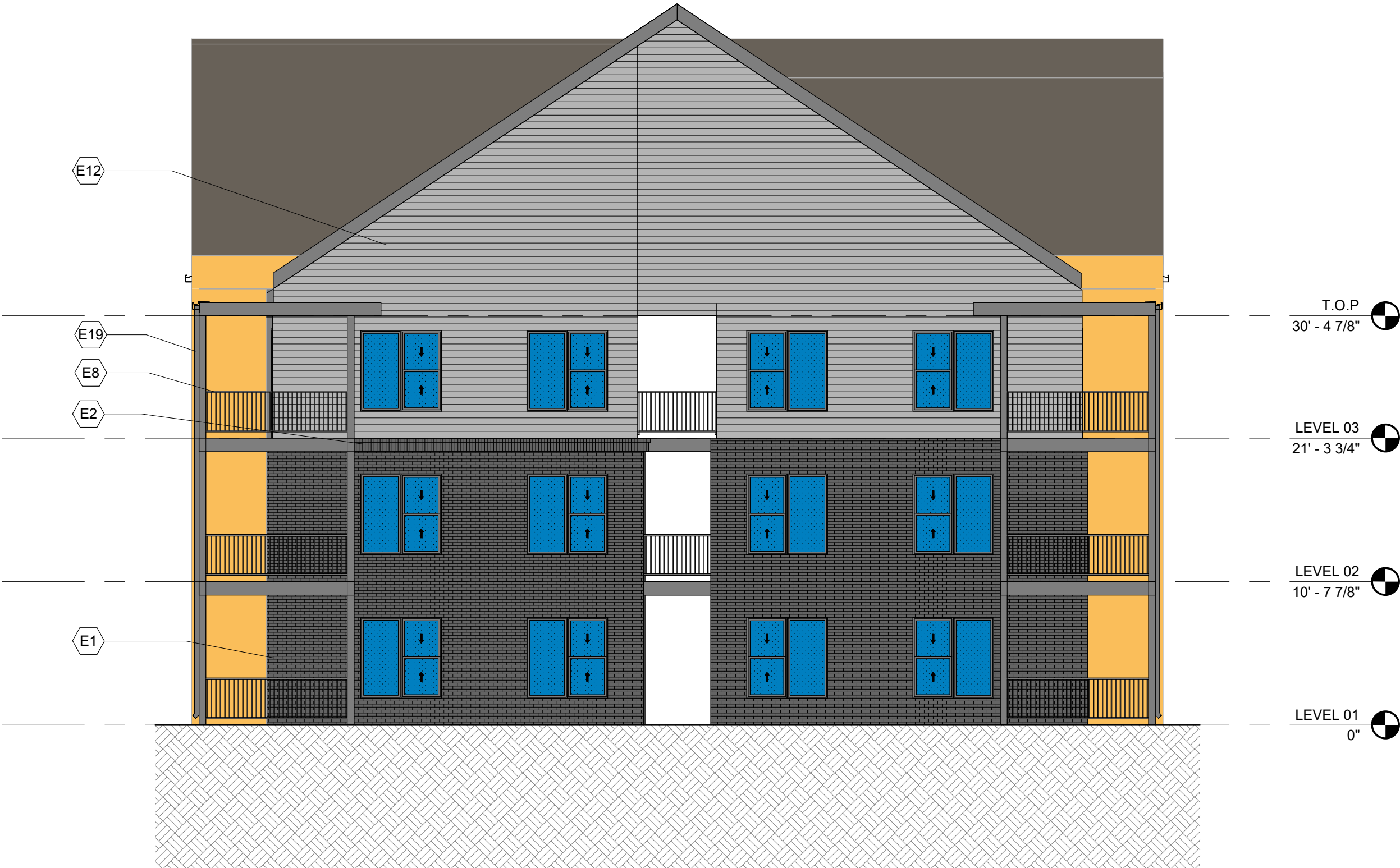
C2 OVERALL ELEVATION - EAST - BUILDING 1 SCALE: 1/8" = 1'-0"
