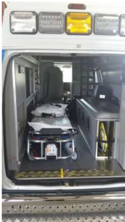
This is the rear entry patient loading door and patient care compartment. As you can see the cot mounting bracket is attached to the wall of the ambulance.
