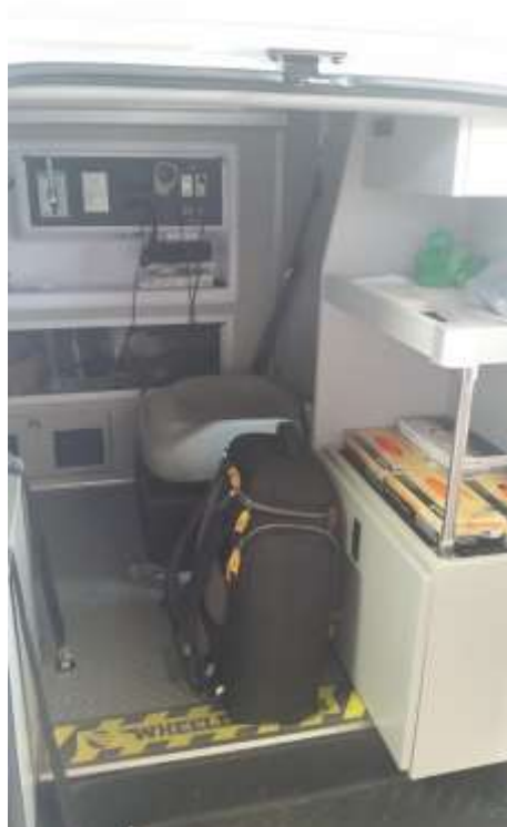
This is the side entry door. The size of the compartments for storing medical equipment is very tight and some of the equipment is not able to be secured in a compartment.
